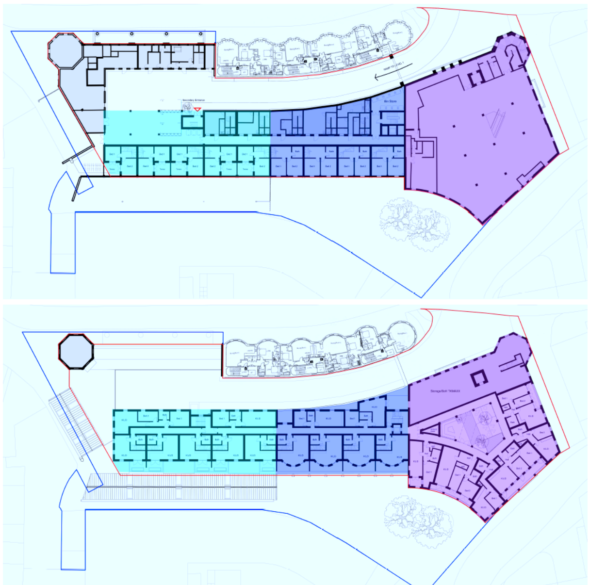
Fig. 3 (upper). Proposed First Floor. | Fig. 4 (lower). Proposed Second Floor Southern End (light blue); Central Section (mid blue); Northern End (purple)
